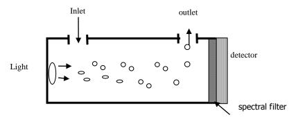
Basic mathematical model: A majority of both organic and inorganic polyatomic gas have specific absorptive wavelength in infrared region. It observes Lambert-Beer Law formula I= I0e-kpl when infrared light is coming through. Light absorption intensity "i" can be described as i=I0-I= I0 (1- e-kpl). I0: intensity of incoming ray. I: transmitting beams. I :thickness of gaseous medium. p: gas concentration. k: absorption coefficient.
